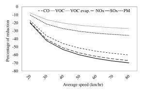
Fig. 8 Percentage of reduction of trucks emission factors comparing with BAU case are affected by average speed.
