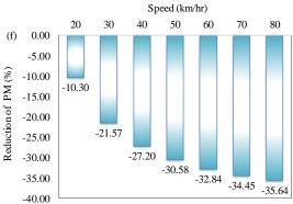
Fig. 7 Effect of increasing speed to reduction of trucks emission factors
